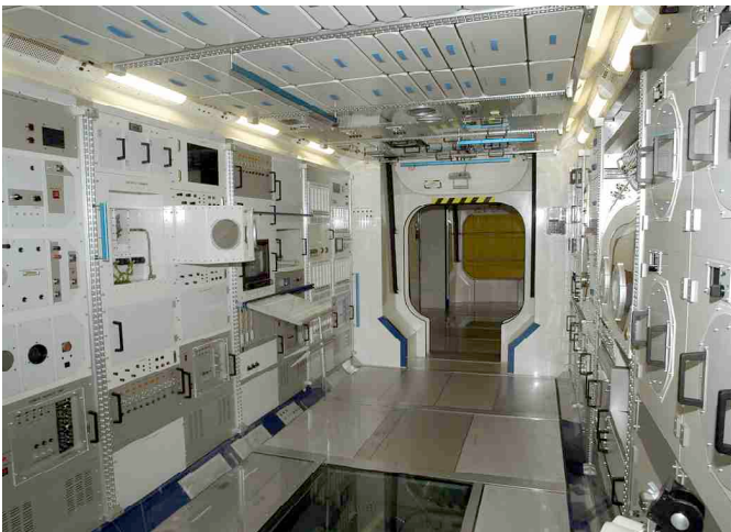
Figure 23 shows the half folded-workstation in a module mock-up. The workstation can be fully folded back to the rack, but also deployed the intrusion into the main passage way in the center of the module is minimal.
