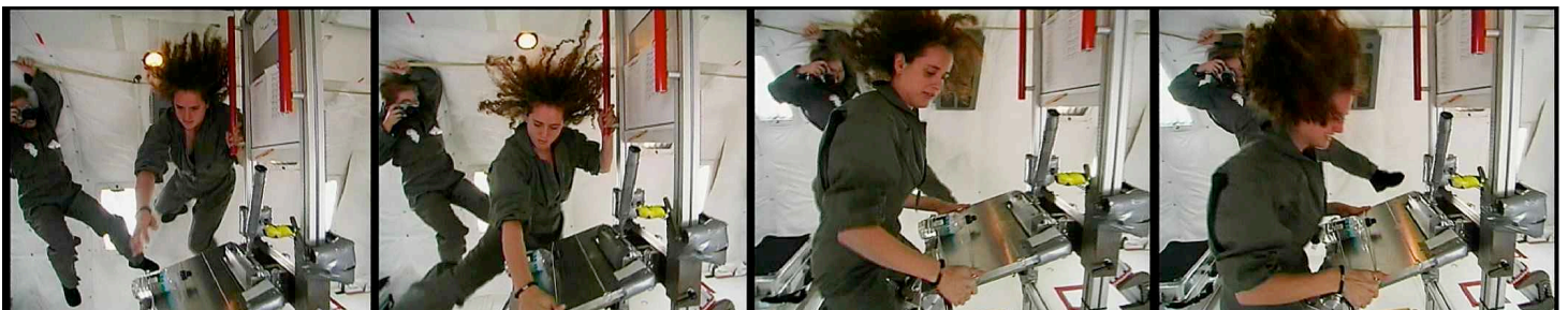
Figure 6: The four images show a video sequence of ingressing the workstation during a parabolic flight. Pictures are taken from a video in half a second intervals, resulting in a total of 2 seconds from approaching the workstation to being fully stabilized and restrained.
