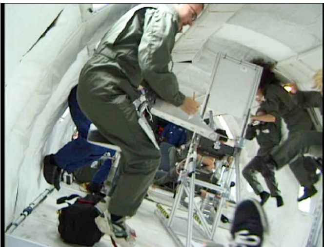
Figure 15 showing the author using the workstation in free-floating mode during a parabolic flight. Note that the seat plates and telescopic arm have not been adjusted and still allow good short-term or ‘stop-and-go’ use of the workstation. Unfolding and egress took less than 10 seconds without adjusting the telescopic arm and without previous training.
